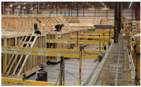
As the walls were being built on the jig, the sheetrock was applied to one surface. This takes a little getting used to at first, seeing a home being built from the inside out. But then the advantages become evident; being able to tape the backsides of sheetrock seams for more strength, and the ability to glue the wall insulation into place so it will never shimmy down. They’ve really thought this through.
